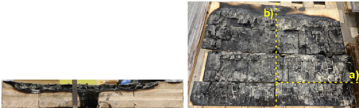
b) Cut in the middle of the CLT panel.
