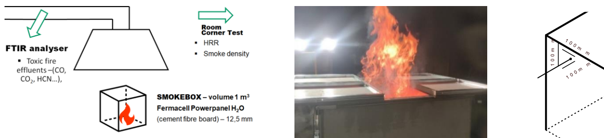
Fig. 1. Schematic view of the experimental setup (left), Smokebox test with 33 % of ceiling open (center), interior thermocouple location (left).
